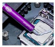
**CryoFuze Thermal Paste**
