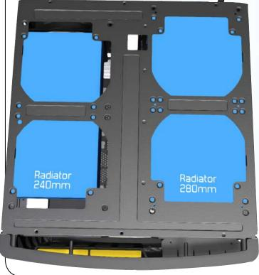
Maximum radiator configuration: 1x240mm, 1x280mm and 2x120mm radiators simultaneously.
